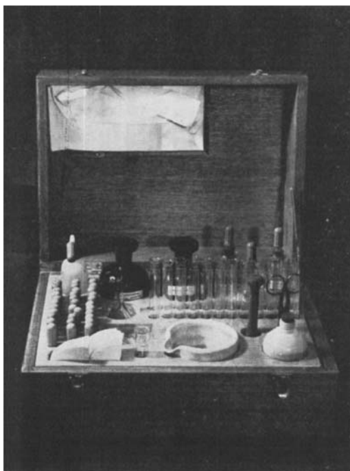
Fig. 1.—Alkaloid testing kit. At rear: Water wash bottle (100 ml.); chloroform containing N /20 ammonia (250 ml.); chloroform (250 ml.); 2 N sulphuric acid with calibrated dropper (100 ml.); Mayers reagent (50 ml.); silicotungstic acid solution (50 ml.); Center: Droppers with cotton wool filter plug (30); 2 in. funnel; 5 in. × 1/2 in. test tubes (24); 1 in. × 1/4 in. test tubes (several dozen). Front: Folded 11 cm. filter papers (24), 3 in. × 3/4 in. test tube calibrated to measure 10 ml.; 3 1/2 in. mortar; pestle; scissors; sand (250 ml. bottle).
